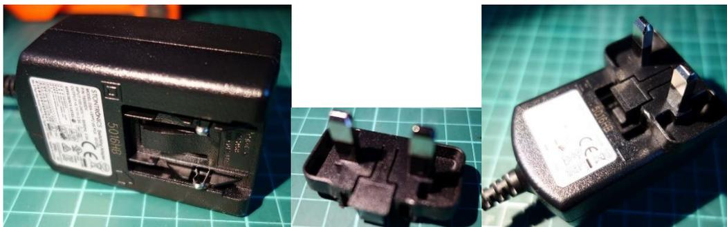
Glue the two 3D printed fillers to the power adapter.
