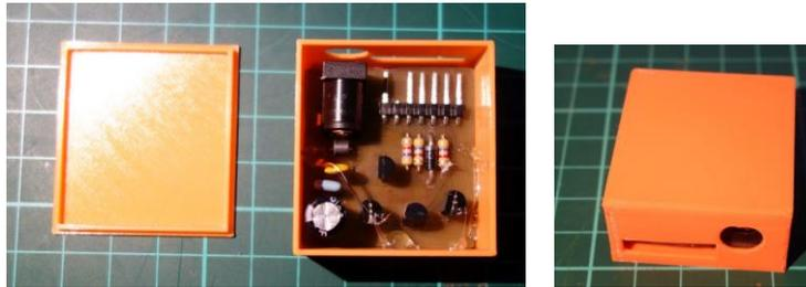
The RPi PSU 5V cable will be cut ~ 10cm from the microUSB connector and a 10cm of bifilar cable will be soldered with the DC power jack at the other end (used to power the control module).
