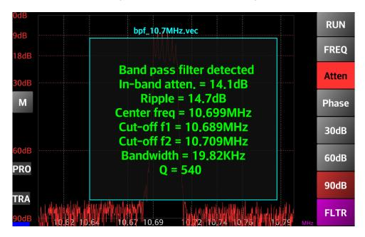
The application can automatically detect (in most situations) the filter type (low pass, band pass, band reject or high pass), adjusting the calculated parameters accordingly. Please be aware that this is still an experimental feature, so it may fail with some filters. Click on the data box to remove it from the screen.
