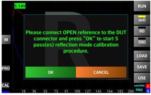
A progress message will be displayed. When the OPEN calibration is completed, remove the OPEN calibration reference from the DUT connector. For the miniVNA Pro, connect the SHORT (0 ohm) calibration reference to the DUT connector as shown in the following picture and press the "OK" button again.
