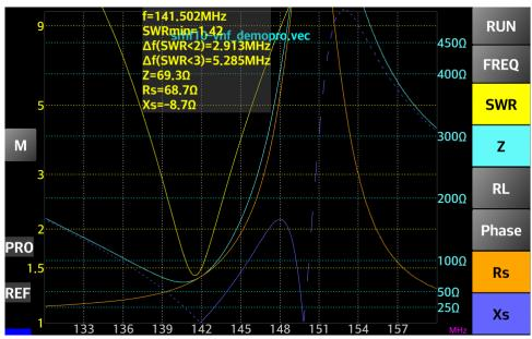
Besides the values for the selected parameter values, the bandwidth ( $\Delta f$ ) for a SWR < 3:1 and for a SWR < 2:1 will be displayed too. If minSWR is > 3:1, then the bandwidth value will not be displayed.
