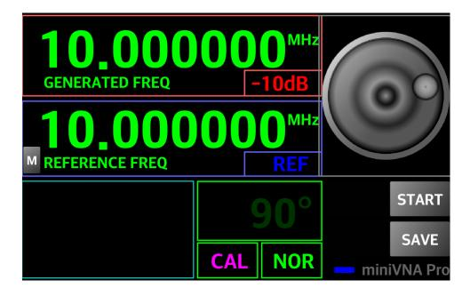
To calibrate, use a very well calibrated frequency meter connected to DUT (miniVNA Pro without extender or miniVNA standard) or TX (miniVNA Pro with Extender). The available frequency range is the one supported by your miniVNA model (0.1-180 MHz for miniVNA Standard, 0.1-200 MHz for Pro without Extender and 40-1500 MHz for Pro with Extender). In this example, the miniVNA will be calibrated using a 10 MHz reference.
