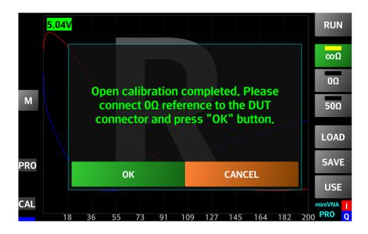
A progress message will be displayed. When the SHORT calibration is completed, remove the SHORT calibration reference from the DUT connector. Then, connect the LOAD (50 ohm) calibration reference to the DUT connector as shown in the following picture and press the "OK" button again."
