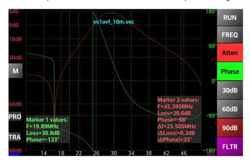
Long press on the "Atten" button to automatically measure the bandwidth at a specific attenuation.
