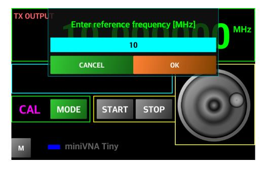
Enter the reference frequency in MHz and press "OK". Reference frequency will be displayed. Start LIVE mode and change the frequency with the tuning knob till the generator output exactly the reference frequency, then press SAVE.
