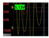
The voltage is displayed with black characters on a colored background. The color of the background depends on the battery voltage as follows:
