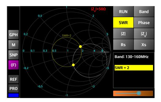
• **Phase** – if this button is pressed, it will change the phase between -180° and +180° using the slider (step 1°). The points on the Smith Chart where the Phase has the selected values are marked with a green dot;
