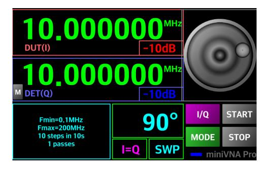
To set the SWEEPER (SWP) parameters long press on "MODE" button when in SWP mode or press the area containing sweeper configuration data in the lower left part of the screen. An overlay will be displayed which will help you to set the parameters values as follows:
