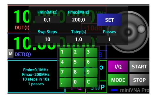
After you enter all the parameters press "SET" button to save them for future use. Values are stored in the configuration file. Now you just have to press "START" button in order to start the Sweeper. To stop it at any time, even the sweep cycle is not ended, just press on "STOP" button.
