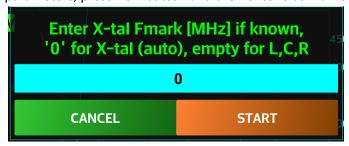
Press START button. The range 1-60MHz will be scanned in 1MHz intervals. Because of a very sharp characteristic of an x-tal, is not possible to do a single scan for the whole range. When the approximative resonance is found by a sharp minimum for the Xs, another scan will be made on a short interval around that frequency. At the end the reflection mode graph and the x-tal parameters will be displayed.
