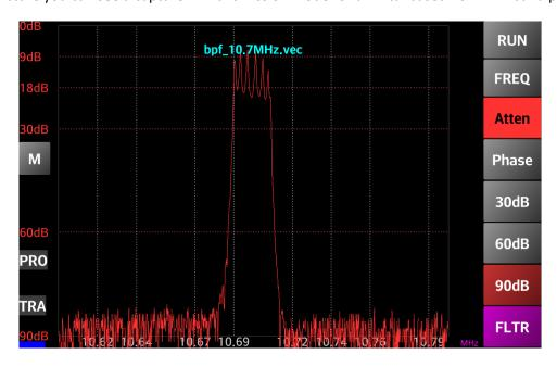
Pressing the "FLTR" button some of the filter parameters will be automatically calculated.
