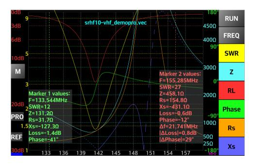
For the second marker, the difference is automatically calculated for frequency and for Loss or Phase (only of the respective parameter is selected using the corresponding button in the right).
