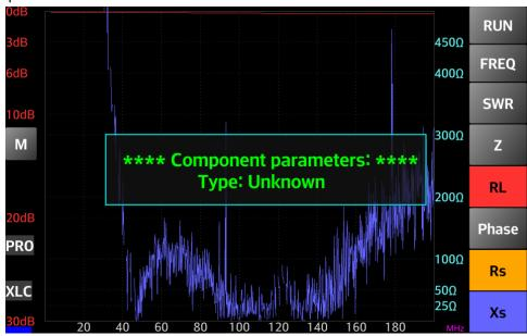
After the capture you can activate the first marker (yellow) in order to display some other parameters for a specific frequency. Where the Xs value is negative, an equivalent capacity is calculated based om formulas from <a href="here">here</a>. Where XS is positive, an equivalent inductance is calculated.
