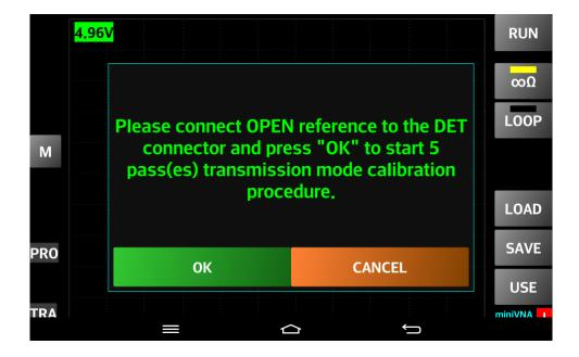
When completed, remove the OPEN reference from the DUT connector.
