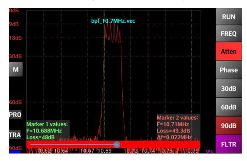
Two markers will be displayed and a red slider in the bottom of the screen. Move the slider left or right do decrease/increase the attenuation to be considered for the bandwidth measurement.
