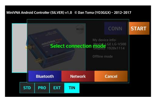
**NOTE:** To use Wi-Fi mode, the miniVNA must be equipped (as an add-on) with a Wi-Fi to serial interface or use a COM port redirector if installing this app inside an Android Emulator (like <u>BlueStacks</u>). <u>The miniVNA's Bluetooth is disabled</u> when it is connected to a USB cable, even if the other end is not connected.
