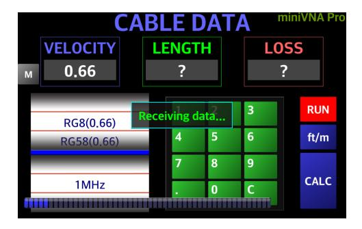
If the cable length is more than a few meters, then the process will be two steps. During the first step, an intermediate value for the cable length will be calculated using the whole available frequency range for that specific miniVNA and the "RUN" button will soon become yellow. When the measurement is finalized, the "RUN" button becomes gray again and the calculated data is displayed.
