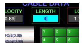
Press the "CALC" button to recalculate the Velocity Factor based on the newly entered cable length. There is no need to run a new capture.
