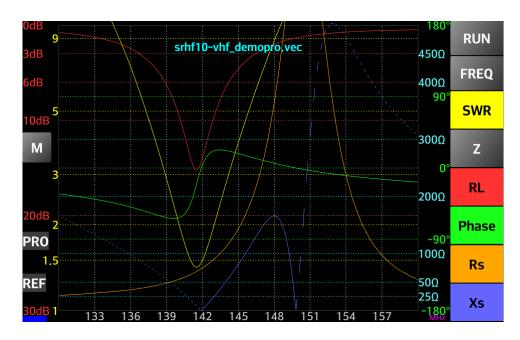
Press a button on the right side corresponding to a parameter to display on the graph. The corresponding graph will be displayed with the same color as the button.
