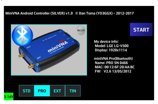
For miniVNA Pro, firmware version will be displayed, together with the battery voltage in the lower left corner. In Tiny case, current battery voltage and internal temperature is displayed.
