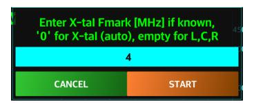
To manually measure X-tal parameters, enter the frequency marked on the X-tal case and press START. A data capture around the marked frequency will start. At the end, you will get the exact resonance frequency and the quality factor.
