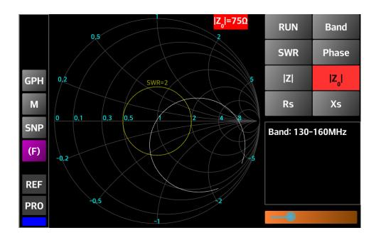
• Rs - if this button is pressed, it will select a value for the real value of the reactance (Rs). The same values as for |Z| are available. The points on the Smith Chart where Rs has the selected value are marked with an orange dot;
