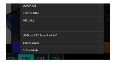
Select your miniVNA from the list (PRO SN 0466 in the picture above) or Offline mode not to connect to the miniVNA. The connection will be established, the background of "START" button goes blue and the Bluetooth symbol will be displayed in the top left corner of the miniVNA "START" screen.
