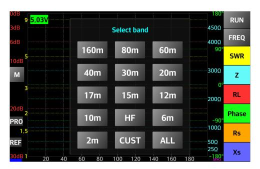
A long press on the "FREQ" button will reset to the full frequency range. Long press on the "10m" button will select the CB (11 meter) band.
