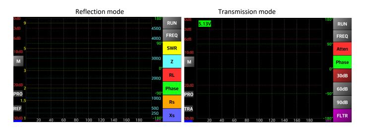
On the left side are the scales for SWR and Loss. On the right side are the scales for Z, Rs, Xs (all in ohms) and Phase (in degrees). Phase is between -180 and 180 for the miniVNA Pro and between 0 and 180 for the miniVNA standard. Xs has an absolute value for the miniVNA standard and a signed value for miniVNA Pro. Negative value for Xs is displayed as a dashed line on the graph.
