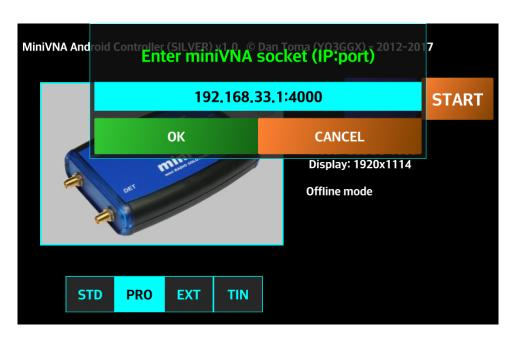
Enter the data in the format IPaddr:port and then press OK. Connection will be established automatically, "START" button background will go green and the Wi-Fi symbol will be displayed in the top left corner of the miniVNA START screen.
