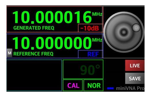
Frequency calibration is completed. Save the frequency calibration data in a calibration file that can be used after a configuration file reset.
