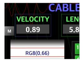
Press the "CALC" button to recalculate the cable length based on the newly entered Velocity Factor. There is no need to run a new data capture. You will be prompted
