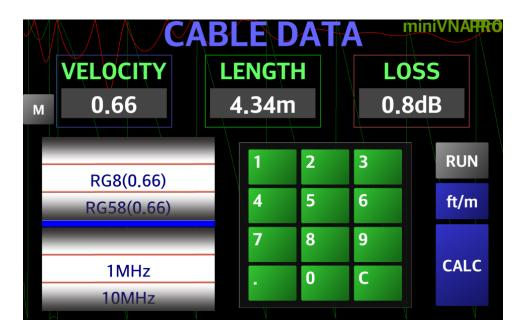
There are 2 graphs in the background. The red graph is for the Return Loss and a green one for Phase. The green graph is used to calculate cable length.
