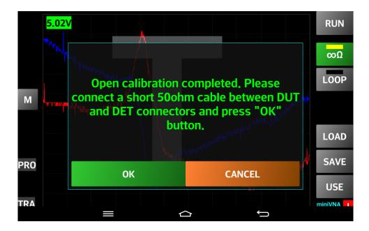
When completed, a confirmation message that the transmission calibration data was captured successfully as shown below. Press the "OK" button to hide the message. The two virtual LED buttons, under the "RUN" button, will become green to indicate that both OPEN and LOOP calibration were performed and a completed message is displayed as shown below.
