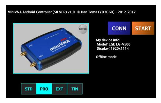
Select the type of device: miniVNA: MiniVNA standard, miniVNA Pro or miniVNA Pro with Extender. Select using a gesture by sliding the picture horizontally or directly press one of the buttons: STD, PRO or EXT. You will get one of the following screens:
