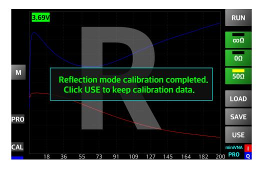
If all 3 steps completed okay, the corresponding buttons on the right side will change to green. In turn, press each of these buttons to see the calibration graphs for OPEN, SHORT and LOAD, which looks like the graphs in the following pictures (i.e., for miniVNA Pro). The large "R" in the background shows the miniVNA is in the reflection calibration mode.
