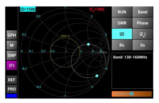
• |20| - if this button is pressed, it will select a value for the reference impedance from the same list as for |Z|. By default, the Smith Chart is displayed for  $|Z0| = 50 \Omega$ , but this value can be changed. The selected value is displayed in the upper right part of the chart (with red background).
