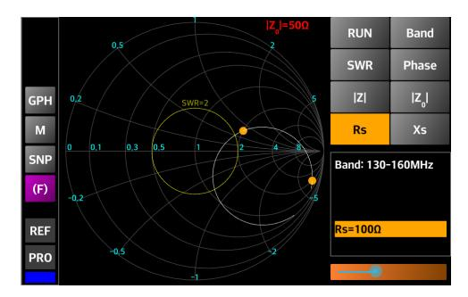
• Xs - if this button is pressed, it will select a value for the imaginary value of the reactance (Xs). The same values as for |Z| are available. The points on the Smith Chart where Xs has the selected value are marked with a blue dot:
