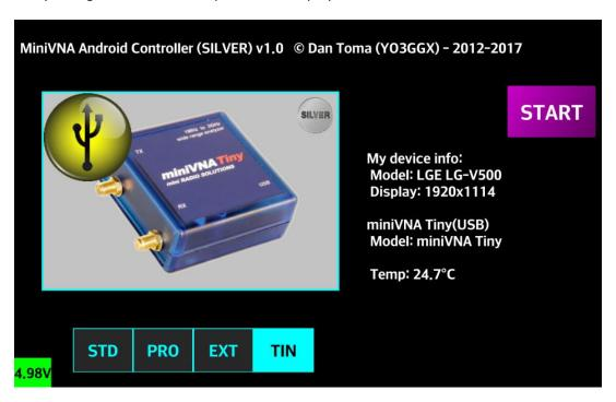
The battery voltage background color will change to yellow when low level and to red when critical. When red, recharging the miniVNA battery is mandatory to prevent battery damage. If your analyzer use an external power, the displayed voltage can be even over 5V.
