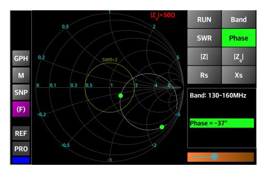
• **Z** - if this button is pressed, it will select one of the following values for |Z|: 25  $\Omega$ , 50  $\Omega$ , 75  $\Omega$ , 100  $\Omega$ , 150  $\Omega$ , 200  $\Omega$ , 300  $\Omega$ , 450  $\Omega$ , and 1000  $\Omega$ . The points on the Smith Chart where |Z| has the selected value are marked with a cyan dot;
