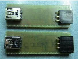
Just insert the module in a piece of transparent heat shrink tube and you're done.
